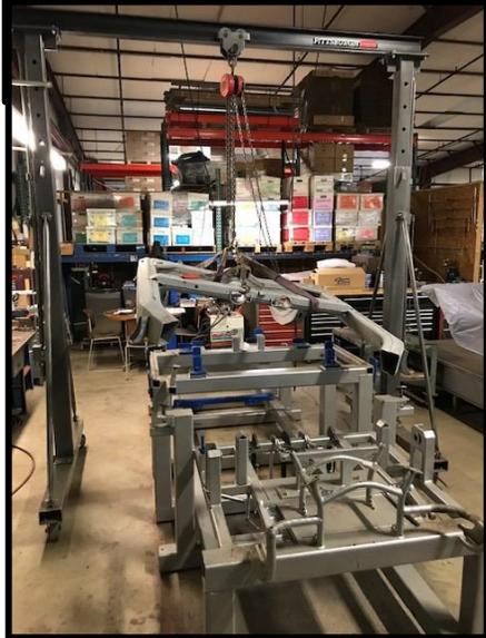
When they came back from sand blasting Roger mounted my frame in his C2 jig and did a thorough inspection. As he had suspected earlier the driver's side frame rail between the transmission cross member and the firewall body mount was  $\frac{1}{2}$  inch low and  $\frac{1}{2}$  inch too far inward as a result of the accident and the poorly done repair job. Roger used his frame table and fixtures to bring the driver's side rail
