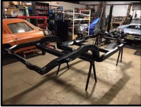
When the frame was finished and all the dimensions were confirmed on the frame jig, the frame was sent out for a second sand blasting and powder coating. It was then bubble wrapped and shipped.
