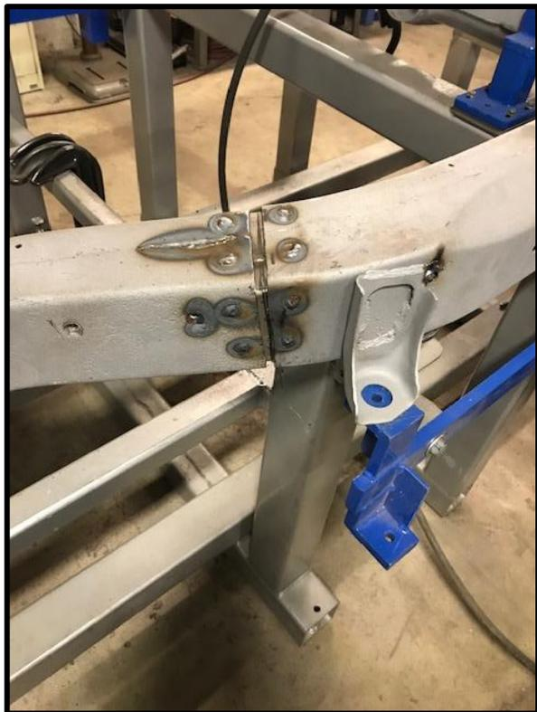
Once both frame sections were mounted in the jig, and the gaps were correct, multiple 3/8 inch holes are drilled in the frame rails and the sleeves are spot welded to the frame rails. As you can imagine there is a sequence to this procedure to insure the front frame section is correctly attached and aligned to the main frame section. Finally, the frame is welded together at the junction of the two frame sections.
