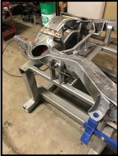
Since my car was going to see plenty of abuse I thought this was a good time to replace the fixed transmission cross member with a removable cross member. This allows easy removal of the transmission without removing the engine.
