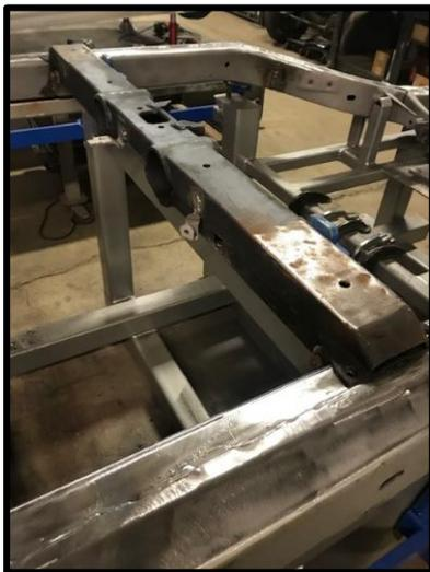
Roger removed the fixed cross member from my frame and welded in the brackets and tabs to make the C3 removable cross member work correctly in my C2 frame. This includes the emergency brake bracket that is specific to the '66 Corvettes. Roger also included the C3 transmission tail shaft bracket for my Muncie 4-speed transmission that works with the new cross member.
